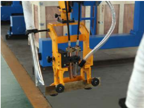
Twin wires with twin arc ( DC+AC )
