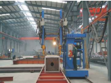
Triple wires with triple arc ( 2DC+AC )
