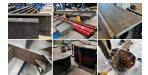
屋面梁，吊车梁，箱型柱，牛腿，铁塔角 Roof beam, crane beam, box column, corbel, iron tower corner
