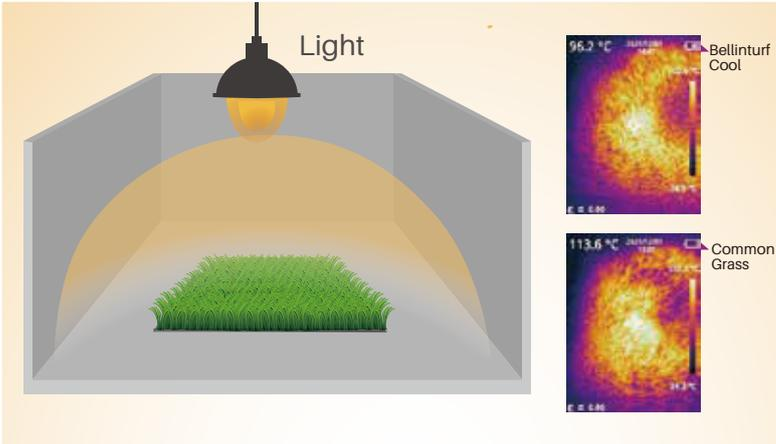
Use a 250W infrared heating lamp to simulate sunlight on the lawn.
