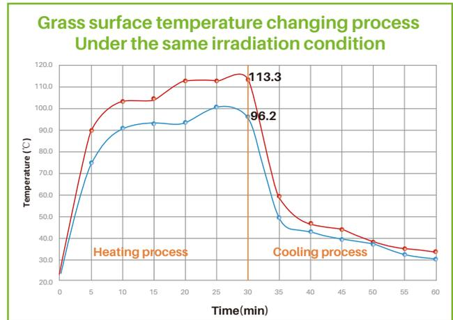
By comparing the temperature curve of ordinary turf and cool grass, it is obvious that the cooling effect of cool grass is good.
