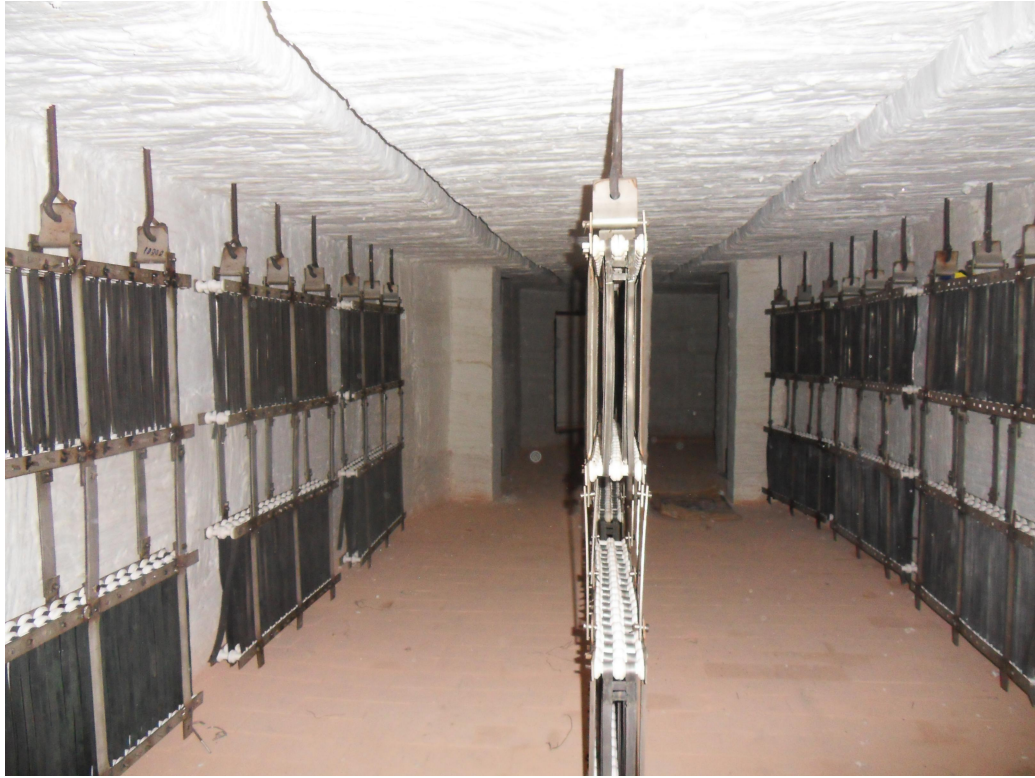
“U”型搪瓷炉结炉电热元件
